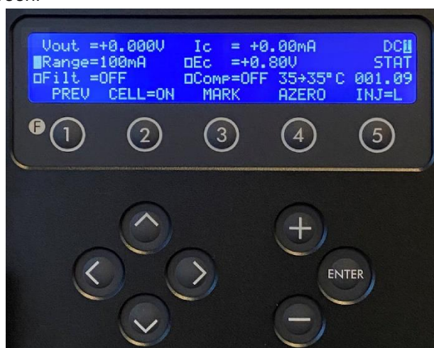
Fig. 5. ROXY Exceed keyboard. The cursor is on 'Range' which allows changes using the value buttons '+' and '-'. The 'Enter' button is only used to confirm changes in potential ( E_c ) and range.
