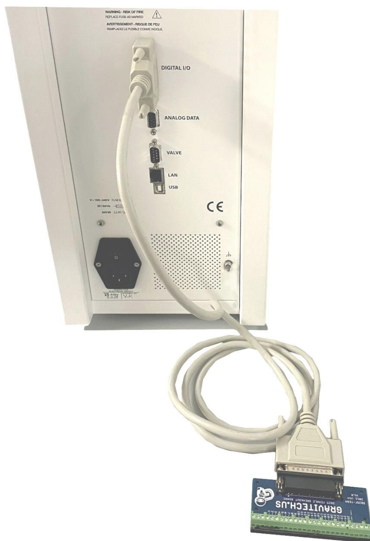
Fig. 57. Left: ROXY Exceed rear panel with I/O screw terminal board installed.
