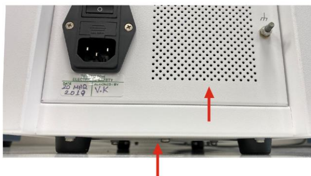
Fig. 2. Location of ventilation holes in the ROXY Exceed (bottom & rear).
